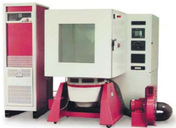
V830-SPA16K shaker system with an environmental chamber.
