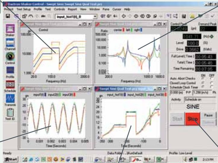
Overlay displays with color traces make it easy to highlight critical measurements.
