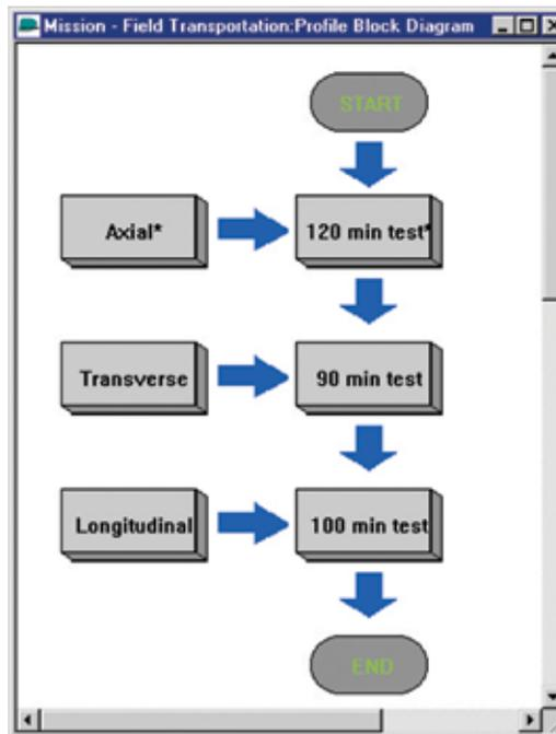
The Profile-Schedule flowchart enables setup and execution of a series of profiles.
