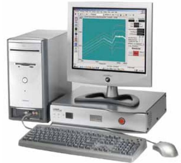
*LASER<sub>USB</sub>* connects to any PC as a USB peripheral. Multiple DSP processors in the *LASER<sub>USB</sub>* handle the control loop in real-time independent of the PC host.
